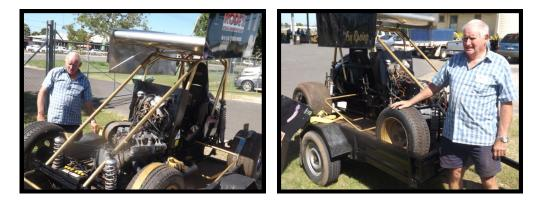
His machine has a 1,000 cc Suzuki motor bike engine which he used to race in the Ilitre sprint car category. Kev still displays the old machine at speedway meets and he keeps up with the 2 litre vehicles which cost twice as much.
